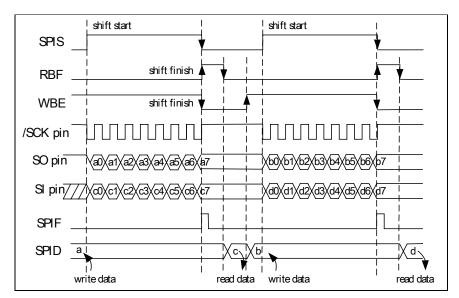
Fig. 5-16 Transmit/Receive Mode (8-bit, 1 word)
